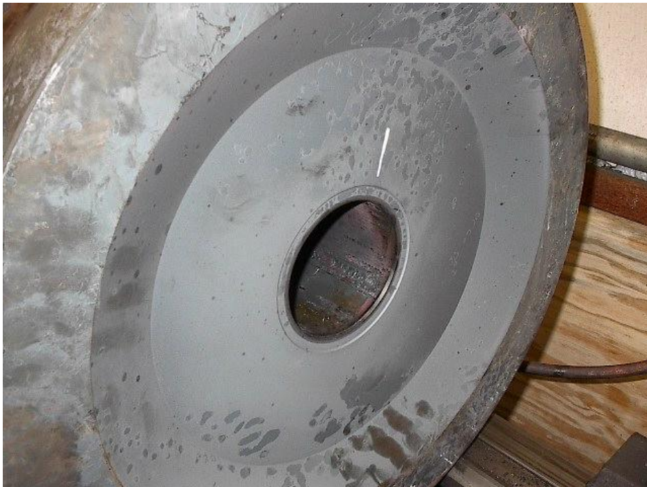
Backseat/breech ID before machining showing galling from stem
