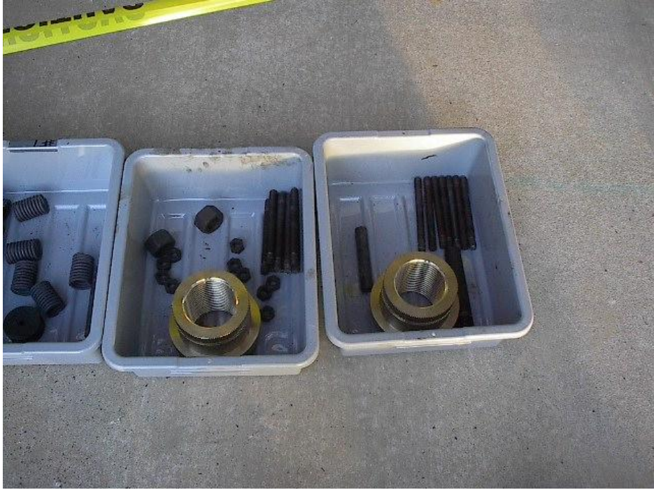
New elevating nuts and studs
