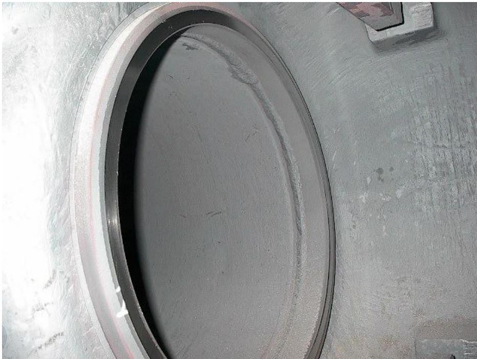
Seat after lapping/polishing
